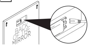
Slide mirror into place and connect power plug to outlet.
