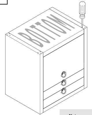
**2.** Attach legs to the cabinet using screws.
